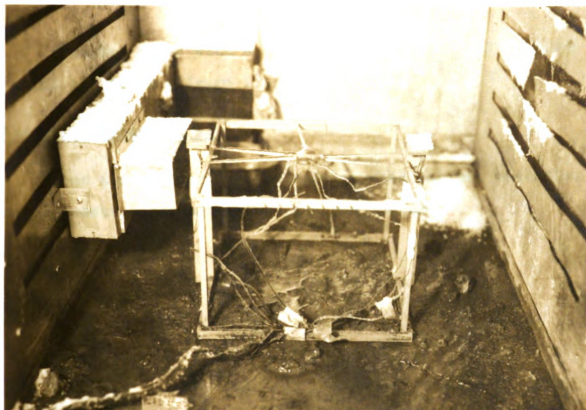
Fig. 7. Leaf stand and leaf after test showing air temperature thermocouples to the left, right and under the leaf.
