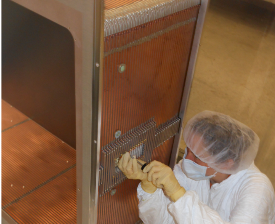
Figure 2.84: Insert window and fingers were put on the window frame of the field cage.
