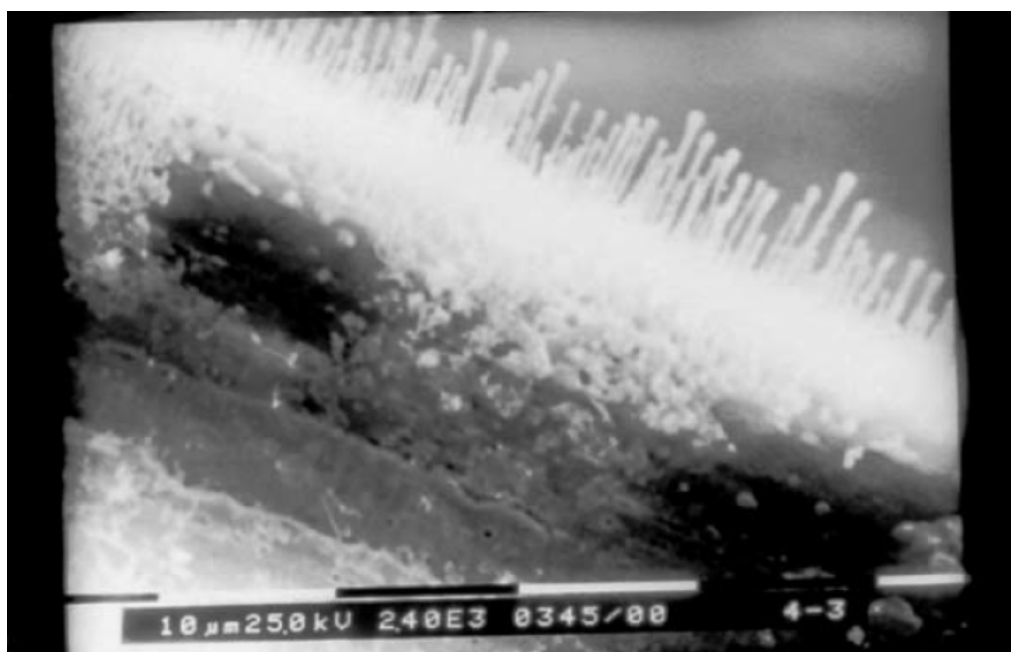
Figure 3.4: Polymers deposit on the surface of an anode wire in \text{CO}_2 /Isobuthane [15]
