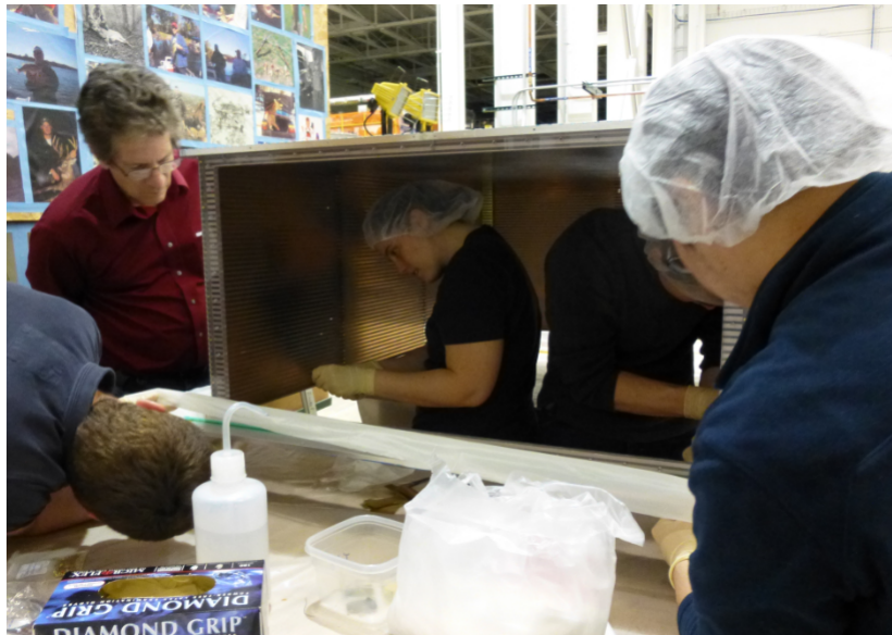
Figure 2.25: Field cage was placed on the support for checking and cleaning the epoxy.
