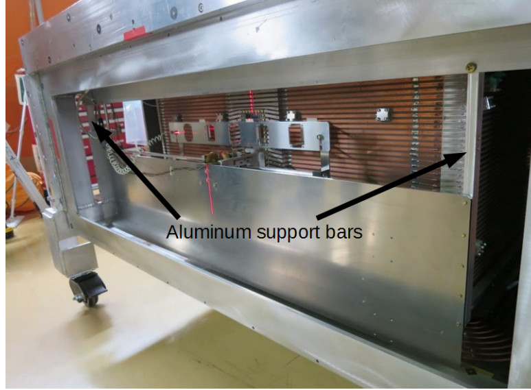
Figure 2.90: The target mechanism is installed onto the S \pi RIT TPC.
