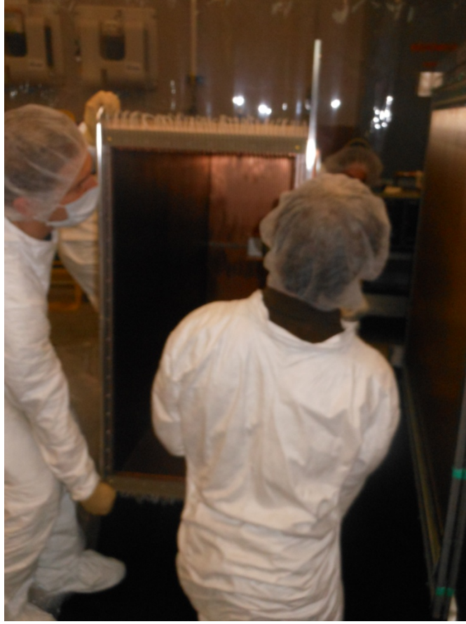
Figure 2.85: Four people lift the field cage and set it on the set screws on the top plate.
