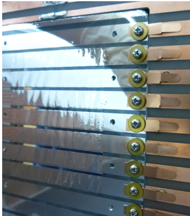
Figure 2.12: The inserted window is put on the front wall of the field cage. The copper fingers provide electrical connections to the strips on the walls.
