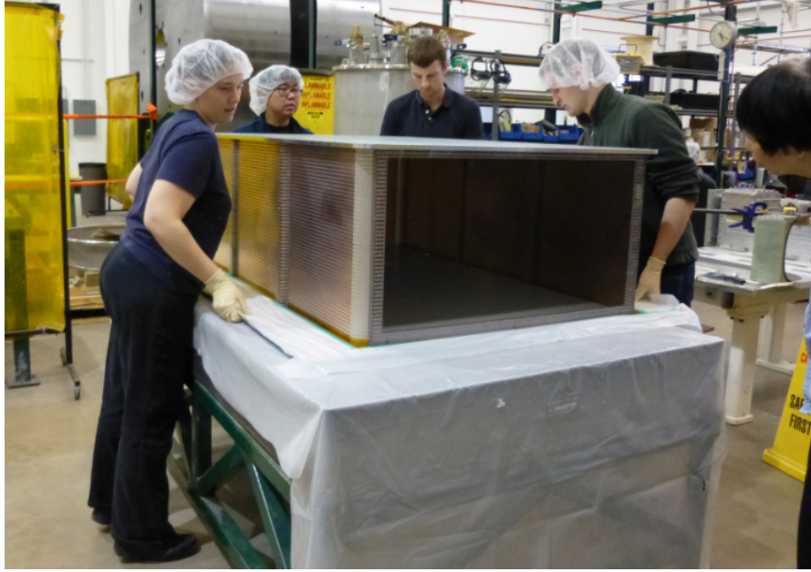
Figure 2.26: Move the field cage to the flat surface to cure for 10 hours.
