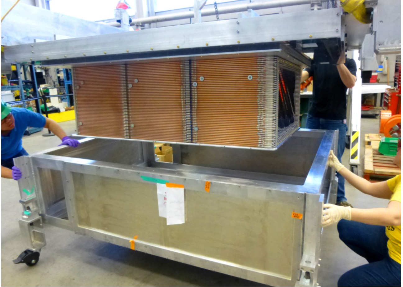
Figure 2.88: Top plate was lowering while people at each corner align the top plate assembly with the enclosure.
