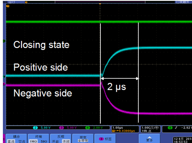
Figure 3.25: The signal from the oscilloscope shows the time of charging a 22\ \text{nF} capacitor to the original voltage of \pm 12\ \text{V} . Blue: signal from the positive side of the capacitor; Purple: signal from the negative side of the capacitor.
