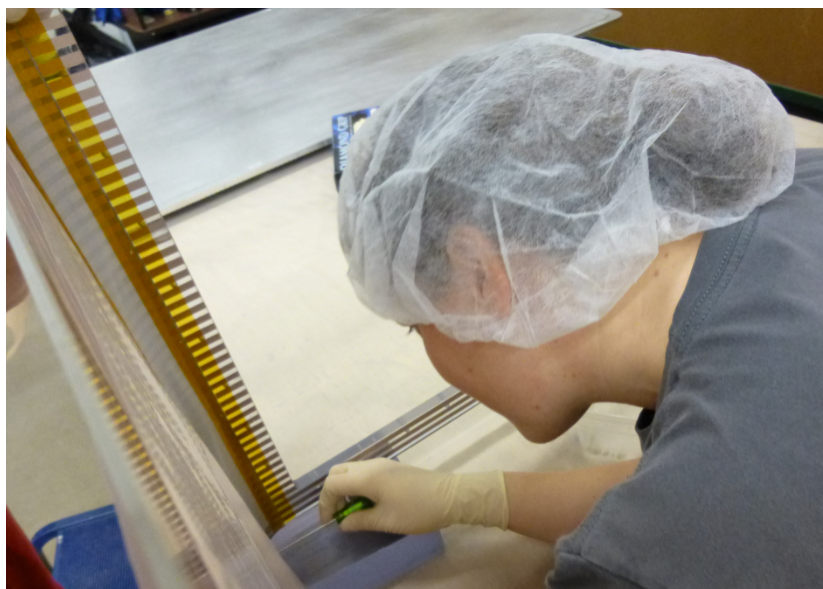
Figure 2.21: Back window frame was attached to the wall of the field cage.
