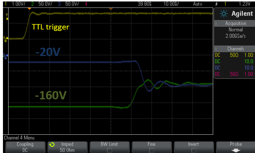
Figure 3.28: The circuit board is tested without connecting to a standard capacitor. The gating grid driver shorts two power supplies together at 45 ns after it is triggered. Blue: discharging signal from the positive side. Green: discharging signal from the negative side.
