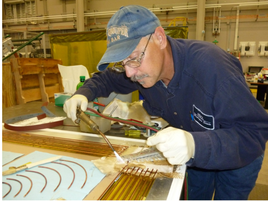
Figure 2.77: A quarter round corner was produced by welding.
