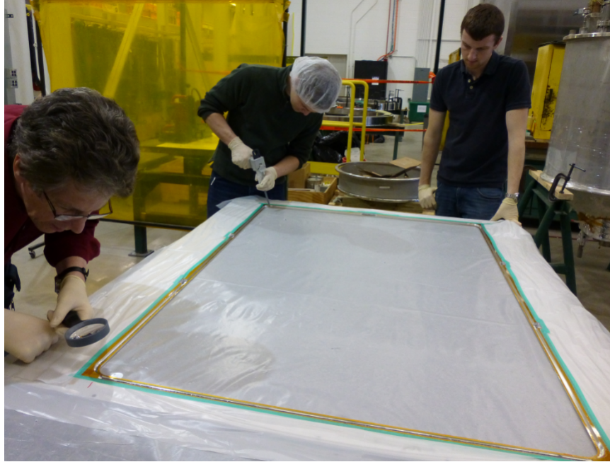
Figure 2.22: Glue excess area on the top perimeter has been masked off with plastic and a Kapton tape.
