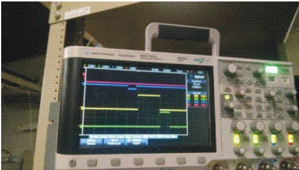
Figure 2.100: A veto signal (blue) occur more than 4 \mu\text{s} before the T-StartScint. The trigger system generate the normal TTL-Open (yellow), TTL-Close (green).
