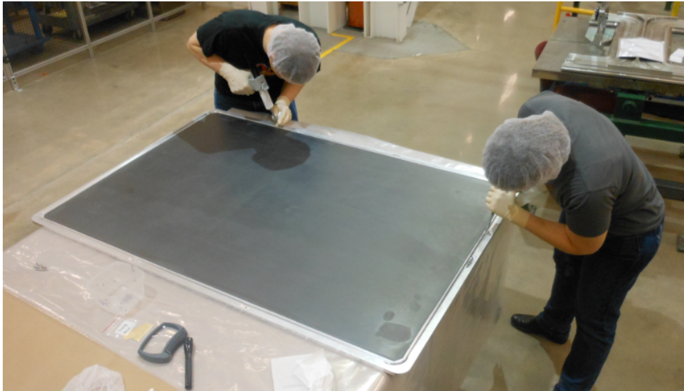
Figure 2.27: Prepare the cathode for gluing.
