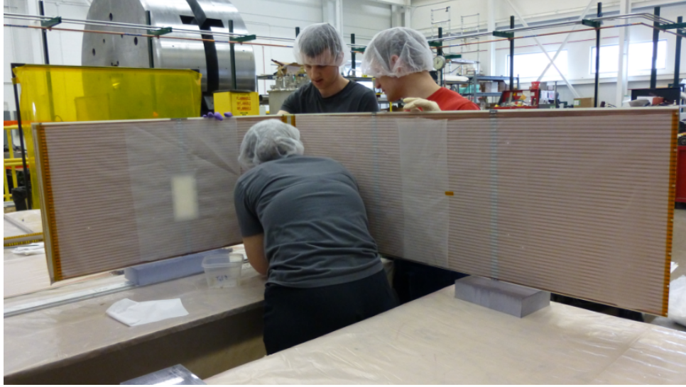
Figure 2.18: Assembling the front and side walls of the field cage.
