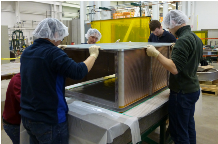
Figure 2.23: Place to the wall of the field cage slowly on the groove filled with beads of Araldite 2013.
