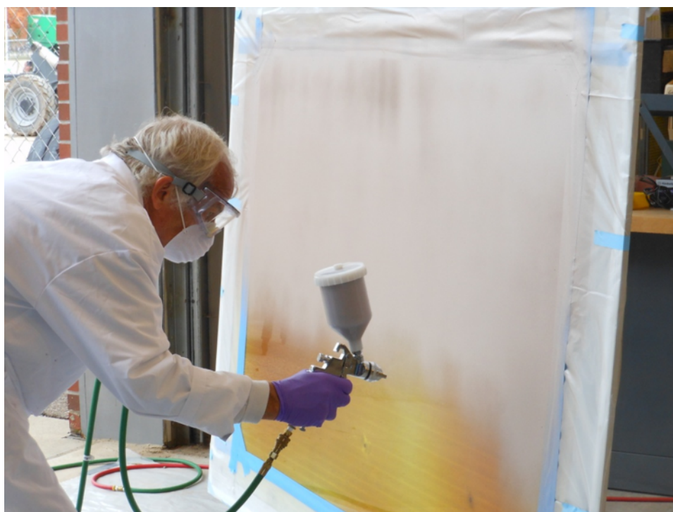
Figure 2.75: Conductive paint was applied at the center of the polycarbonate sheet.
