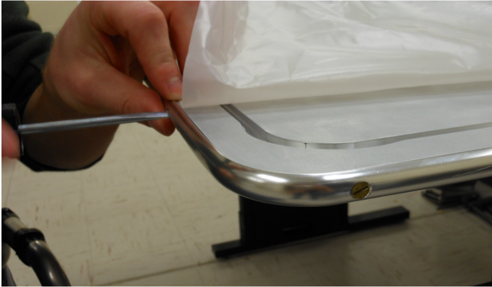
Figure 2.16: Round aluminum edge was attached to the edge of the cathode to reduce a sharp angle.
