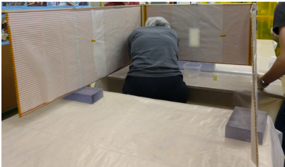
Figure 2.19: Assemble both side walls of the field cage.
