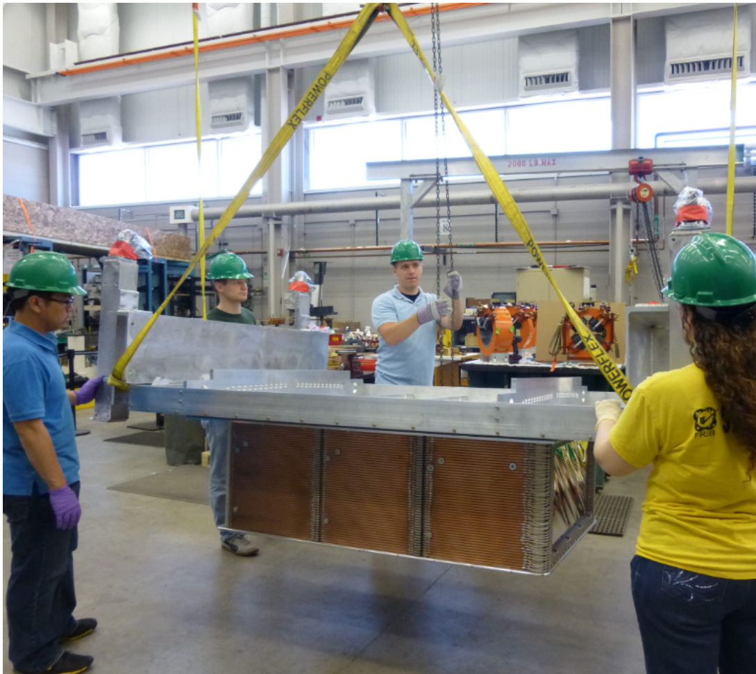
Figure 2.87: Top plate with the field cage attached has been rotated to the position for assembling to the enclosure.
