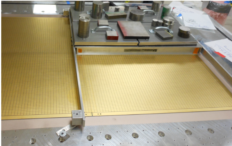
Figure 2.46: Pad-plane PCB is put to the position by the vacuum table.
