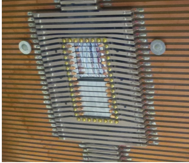
Figure 2.13: The strips on a thin PPTA are connected to the strips on the window frame by copper finger.
