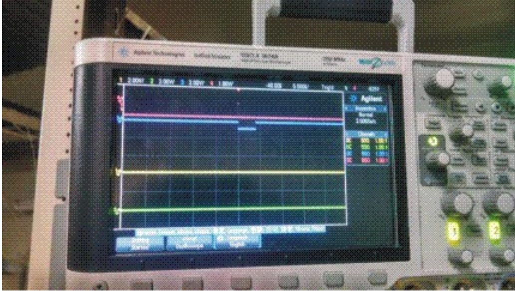
Figure 2.101: There is no generation of TTL-Open (yellow) and TTL-Close (green) when the T-StartScint (purple) and T-Veto (blue) are simultaneous present.
