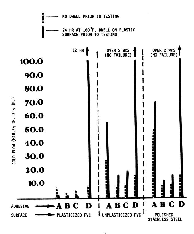
FIGURE 2: COMPARATIVE STUDY OF COLD FLOW IN VARIOUS PRESSURE SENSITIVE ADHESIVES ON PLASTICIZED AND UNPLASTICIZED POLYVINYL CHLORIDE SURFACES. STAINLESS STEEL SURFACE WAS USED AS CONTROL.
