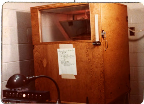
Plate 4. The front view of the sound attenuating chamber used in this experiment. At the top center of the photograph can be seen the plexiglass window and the mirror which allowed an unobstructed view of S during running.
