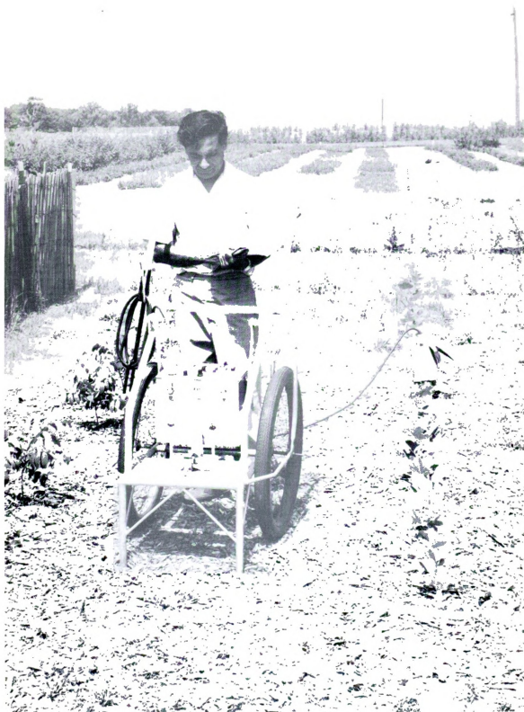
Figure 1. Measurement of soil moisture with Nuclear-Chicago depth neutron probe and portable scaler.
