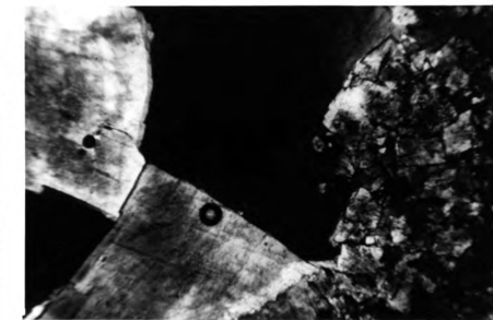
Figure 7c. Extremely coarse-grained baroque or saddle dolomite from the Albion-Scipio field. This dolomite occurs as a void filling. Note curved crystal faces and coarse grain size in comparison to dolomite matrix. Width of field = 2.7 mm.
