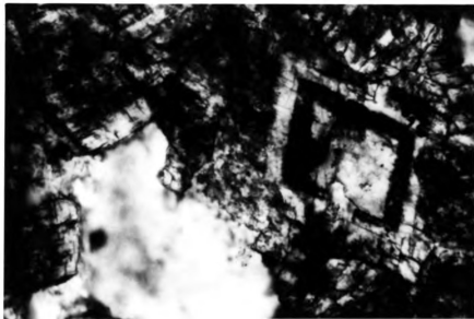
Figure 10d. Ferroan dolomite zone which has been broken by non-ferroan fracture dolomite connecting the core and outer non-ferroan dolomite zone. Width of field = 0.35 mm.
