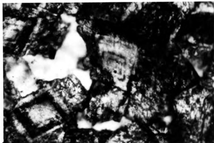
Figure 10b. Stained thin section showing small Fe-rich zones in non-ferroan dolomite cores. Outer zone is ferroan dolomite. Width of field = 0.35 mm.
