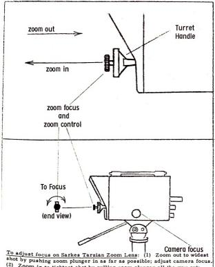
(2) Zoom in to tightest shot by pulling zoom plunger all the way out; adjust zoom focus.
