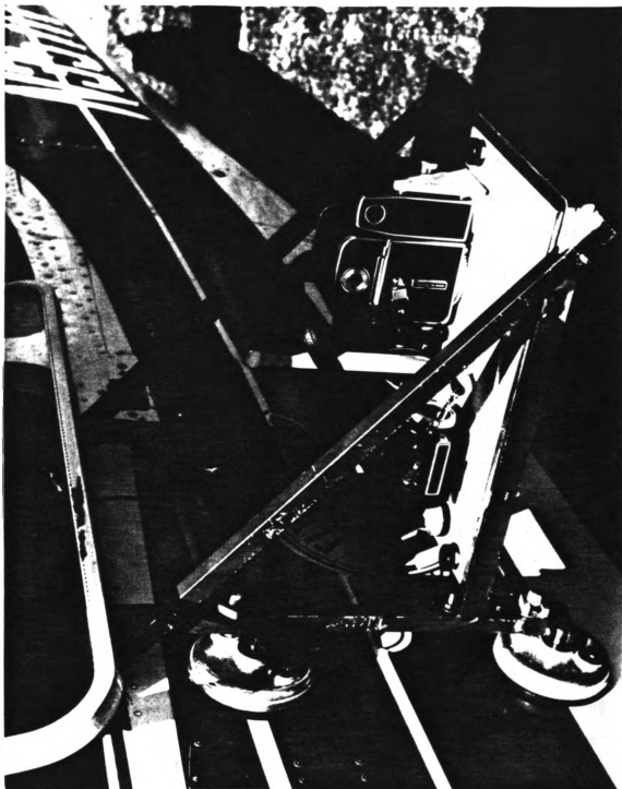
FIGURE 8. Aircraft camera slide-mount with 70mm and 35mm camera systems installed.
