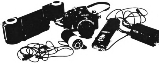
FIGURE 12. Nikon 35mm camera, large motorized back for 250 exposures, battery pack and intervalometer.
