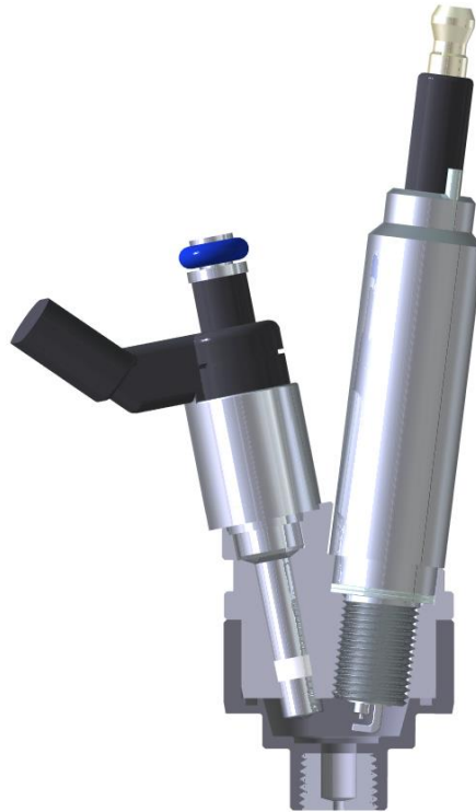
Figure 1-3. TJI assembly: fuel injector, spark plug, pre-chamber adapter body, and nozzle.
