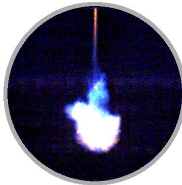
Figure 3-9. Enhanced image at 1.7 ms showing that there is not complete quenching of the jet as it discharges.
