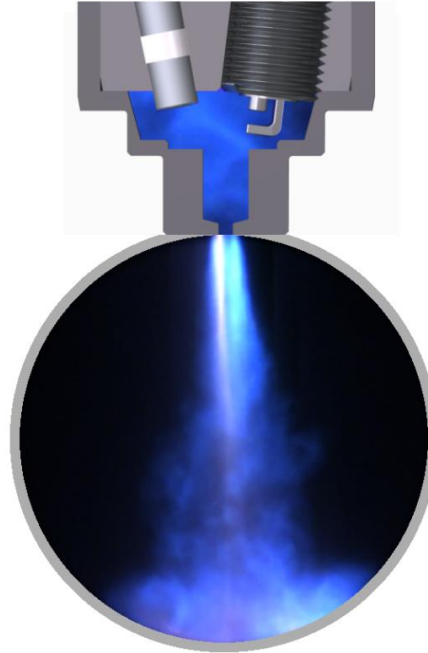
Figure 1-1. Illustration of TJI with a single orifice nozzle
