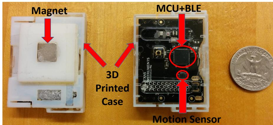
Figure 4.3: The miniature SensorTag device and a customized 3D printed case with an embedded magnet.
