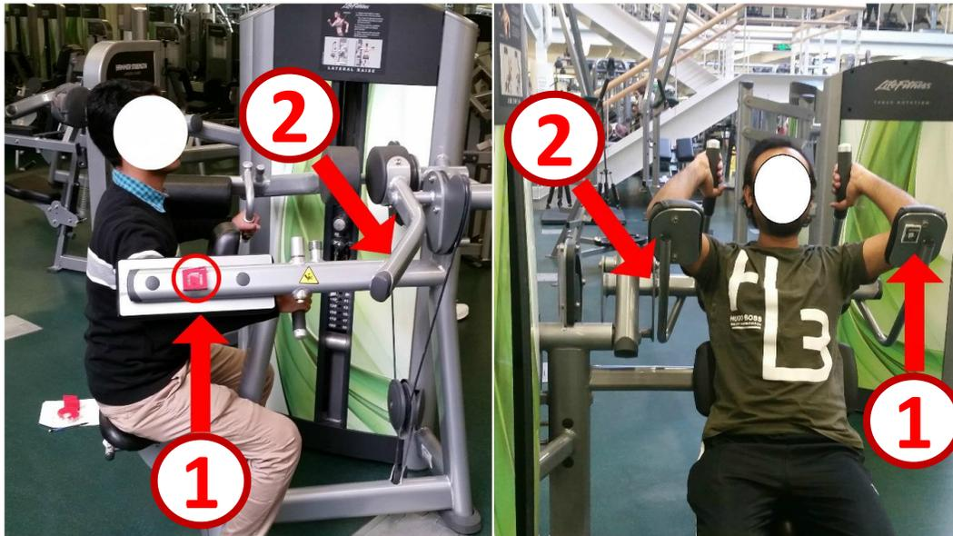
Figure 5.1: The illustration of data collection setup and sensor tag placement using lateral raise machine (left) and seated abs machines (right). Circled 1 and 2 indicate the placement of two sensor tags on each machine.
