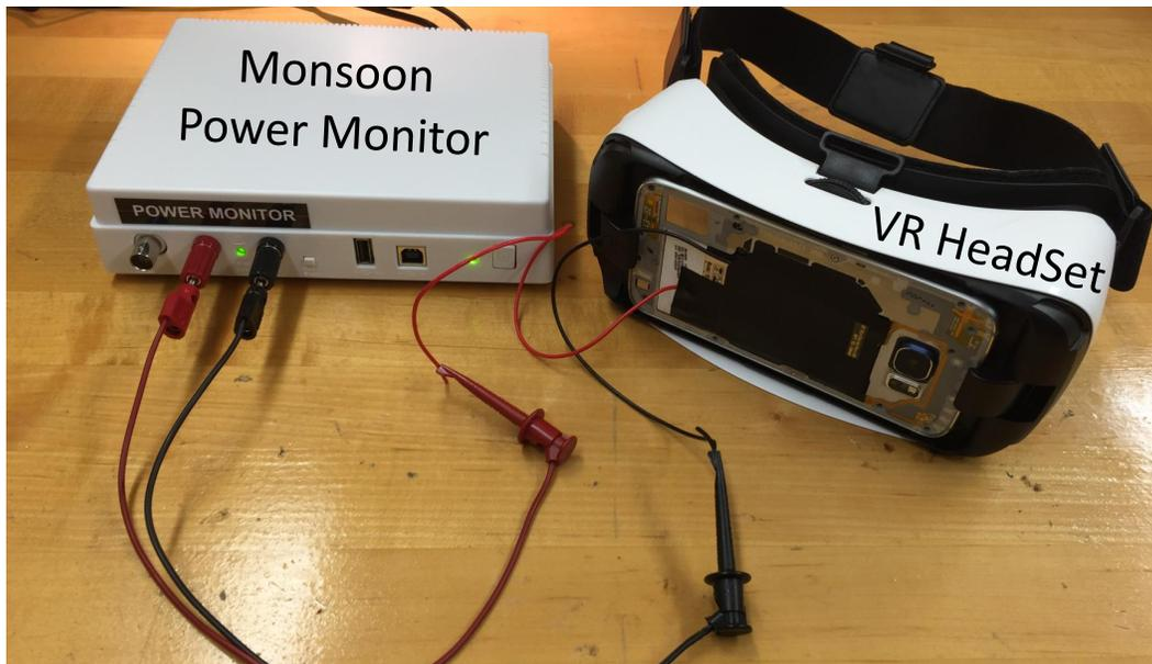
Figure 5.5: Energy consumption measurement setting with Samsung Galaxy S7, Gear VR and Monsoon Power Monitor.
