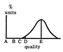
It is also possible that the manufacturer will improve the materials used or the design employed. In this case the distribution might remain unchanged, but the average quality will be improved and fewer units will be in the A to B or B to C range. The average quality has improved from D to E. The mix that companies will actually use between more inspection, better materials and improved design will vary according to their relative effectiveness and cost. Most firm
