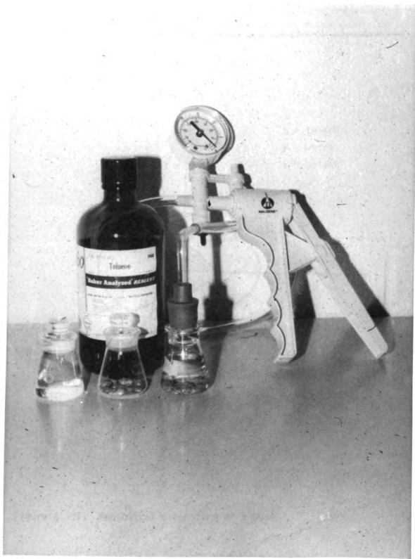
Figure 4.6.1: Pycnometer set-up for specific Gravity determination.
