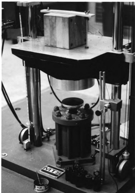
Figure 26. Calibration of Telemetry Wood Block on Shock Machine with Gas Programmer
