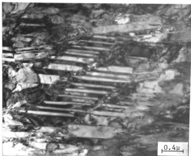
Figure 2.7 Typical transmission electron micrograph showing microstructures of the acicular \text{Ni}_3\text{Sn} martensite.
