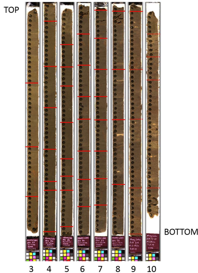
Figure 5.2 Drives 3-10 from the 2014 Hovey Lake, Indiana composite core (Photos by Dr. Broxton Bird, IUPUI, 2014). The core is generally described as very fine sand and silt; a few inclusions of coarse sands and gravels likely indicate periods of flooding. Solid red lines on drives 3—9 (200—1,260 cal yrs BP) indicate where the samples utilized in the pollen diagram were taken. Dotted red lines were outside the timeframe of the study and not included in the pollen diagram.
