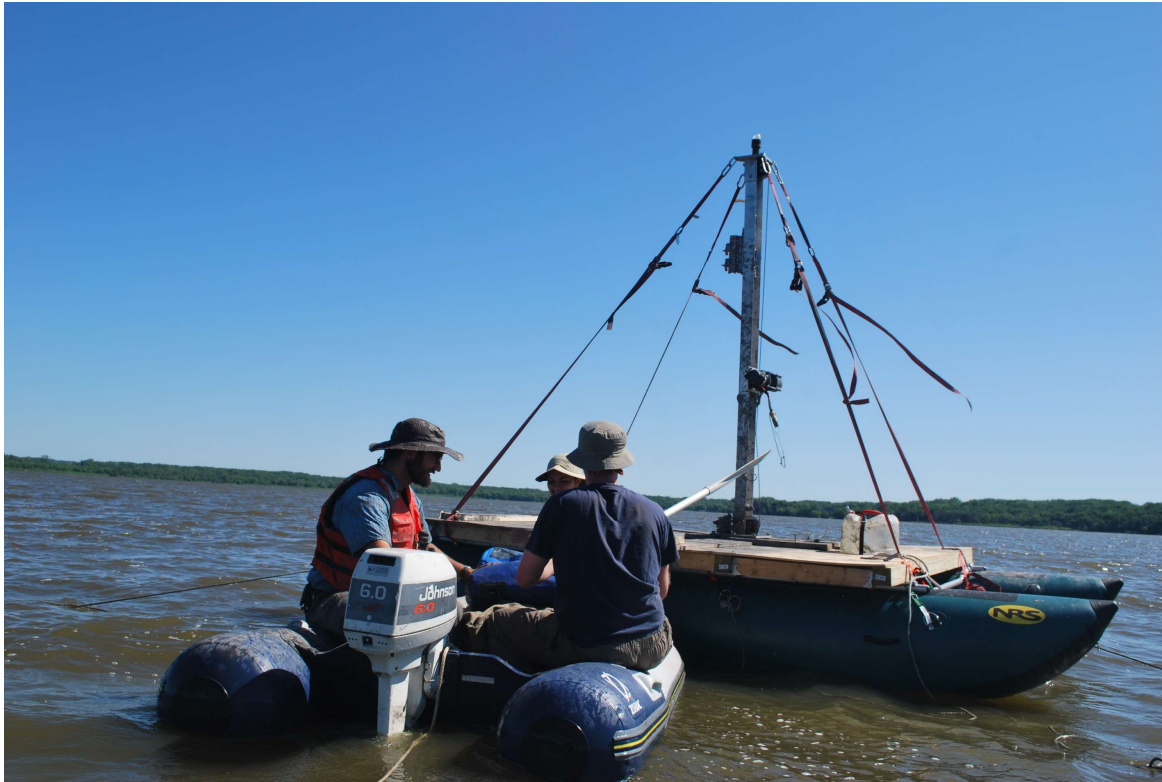
Figure 4.2 A coring platform assembled and anchored on Anderson Lake, Illinois, June 2014 (Photo by Caitlin Clark, 2014). This platform set up was also used at Hovey Lake, Indiana in July 2014.
