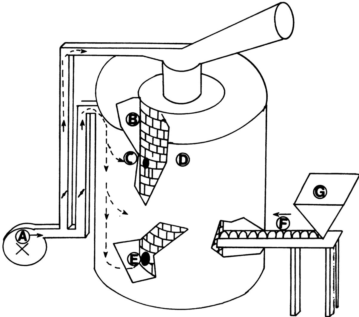
Figure 10. Concentric vortex biomass furnace.
