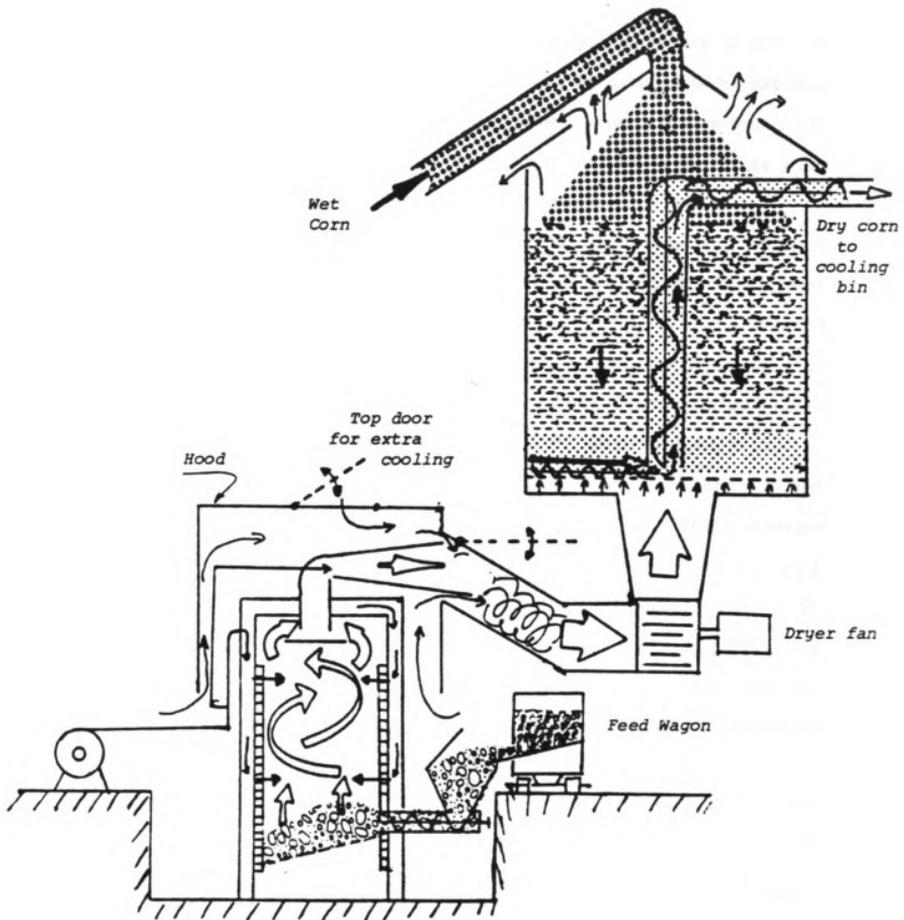
Figure 16. Schematic diagram of Michigan State biomass fired drying system. Source: Mwaura et al., 1982.
