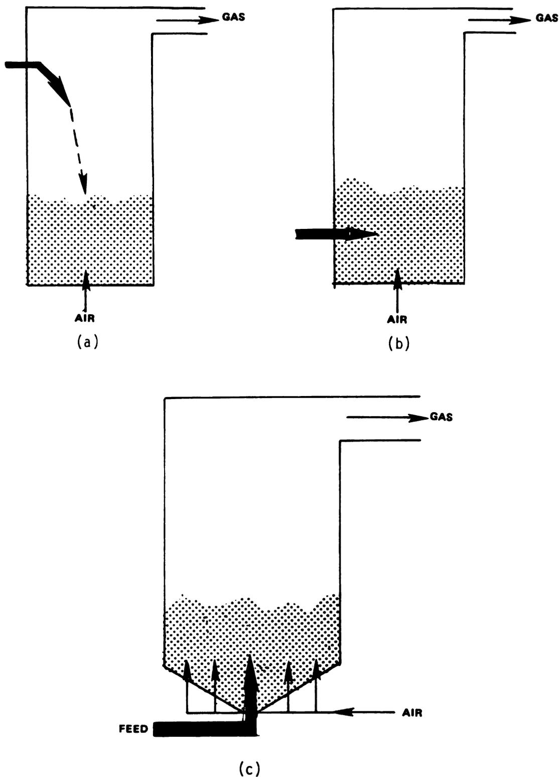
Figure 7. Feed systems for a fluidized bed furnace: (a) top feed, (b) side feed, (c) center feed. Source: Moreno and Goss, 1983.
