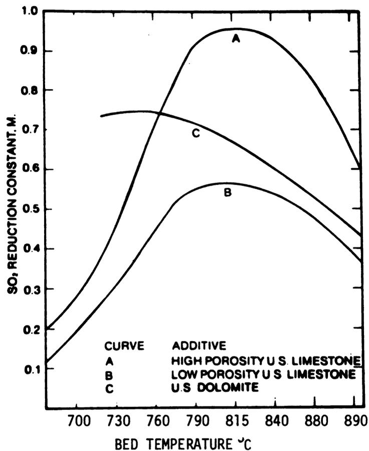
Figure 5. Variation of SO<sub>2</sub> reduction constant M with bed temperature and additive type in a bed 36 inches (91 cm) deep at atmospheric pressure: 6 ft/sec (1.8 m/sec) fluidizing velocity, with fines recycled (from Wallish, 1981).
