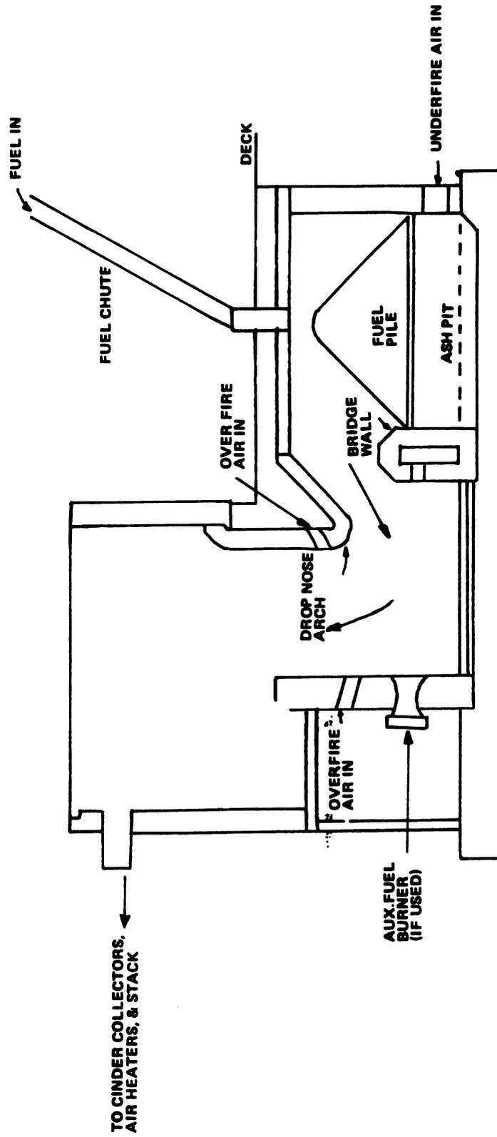
Figure 9. Dutch oven. Source: Levi and O'Grady- 1980.
