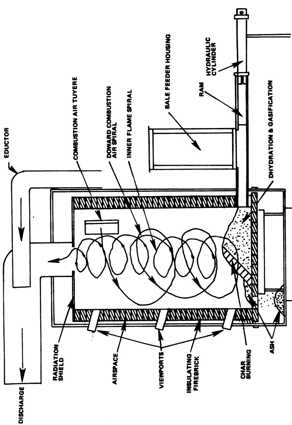
Figure 15. Elevated detail of concentric vortex biomass furnace and ram feeder. Source: Kranzler et al., 1982.
