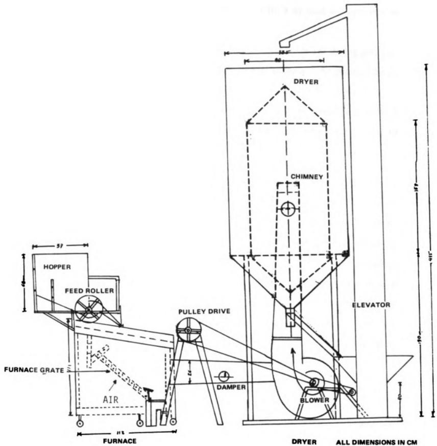
Figure 12. Grate type husk fired furnace coupled with dryer.
