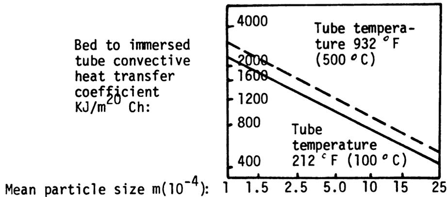
Figure 6: Fluidized bed heat transfer coefficients (from Charagundla & Metrek, 1977).
