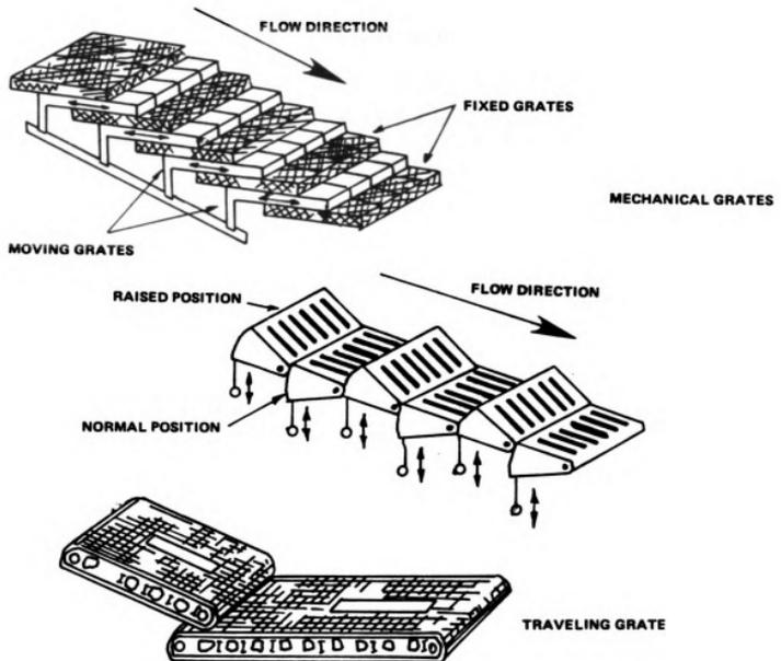
Figure 2. Types of moving grates. Source: Alter and Dunn, 1980.
