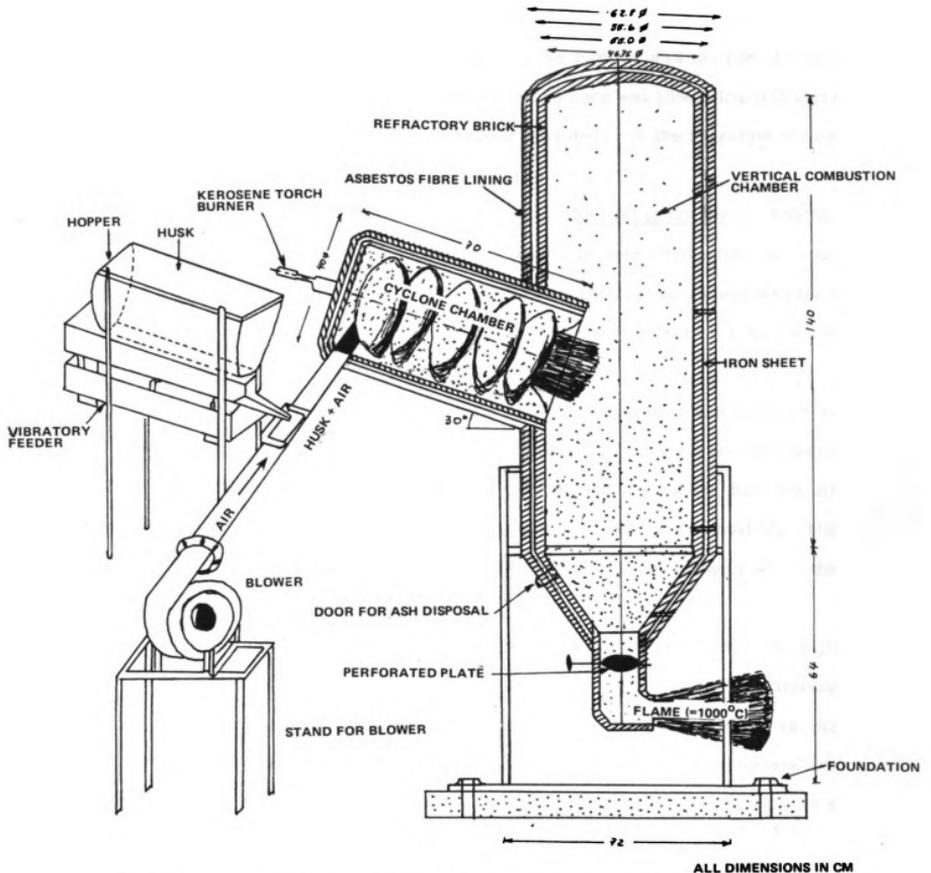
Figure 17. Schematic diagram of a husk fired cyclone furnace.
