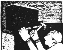
Drawing 1: Where the joists run at right angles to the wall, press short pieces of insulation against the Header — they should fit snugly. Then install the wall and perimeter insulation by nailing the top of each strip to the Sill using the 1/2" X 1-1/2" nailers. Make sure the batts fit snugly against each other, and that you cut them long enough to cover 2 feet of floor as in Drawing 2.
