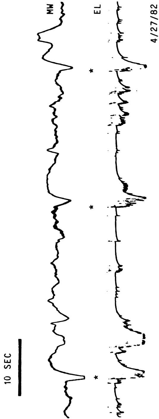
Figure 12. Spontaneous Activity of the Cockroach Nerve Cord as Detected by the EMT.
