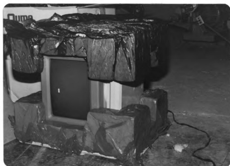
Figure 6. Example of Polyurethane Foam-in-Place Cushion Design 24
