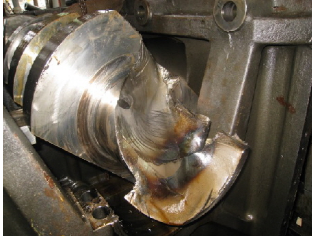
Figure 3.1: A crankshaft with torsional failure [3]
