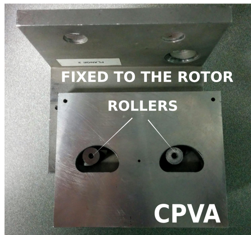
Figure 1.3: The bifilar suspension of a CPVA used as a test specimen at MSU.
