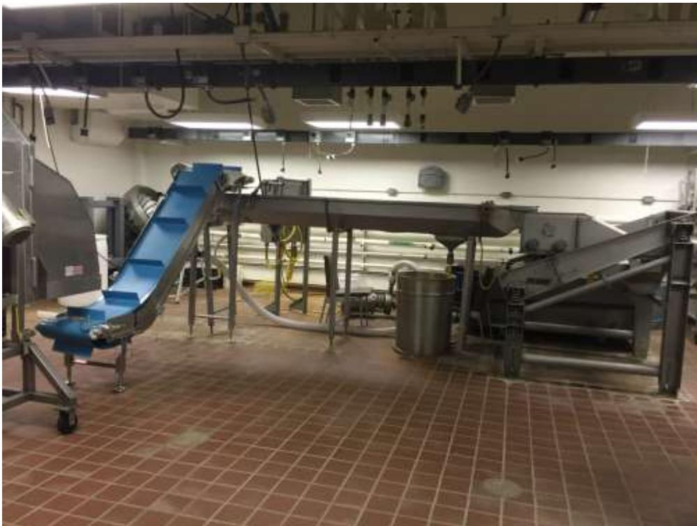
Figure 2.2: Gated flume tank and shaker table
