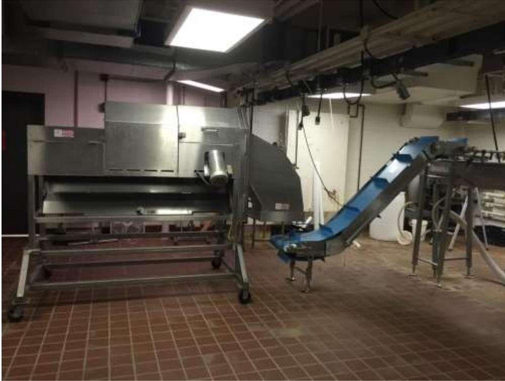
Figure 2.1: Lettuce shredder and step conveyoyr
