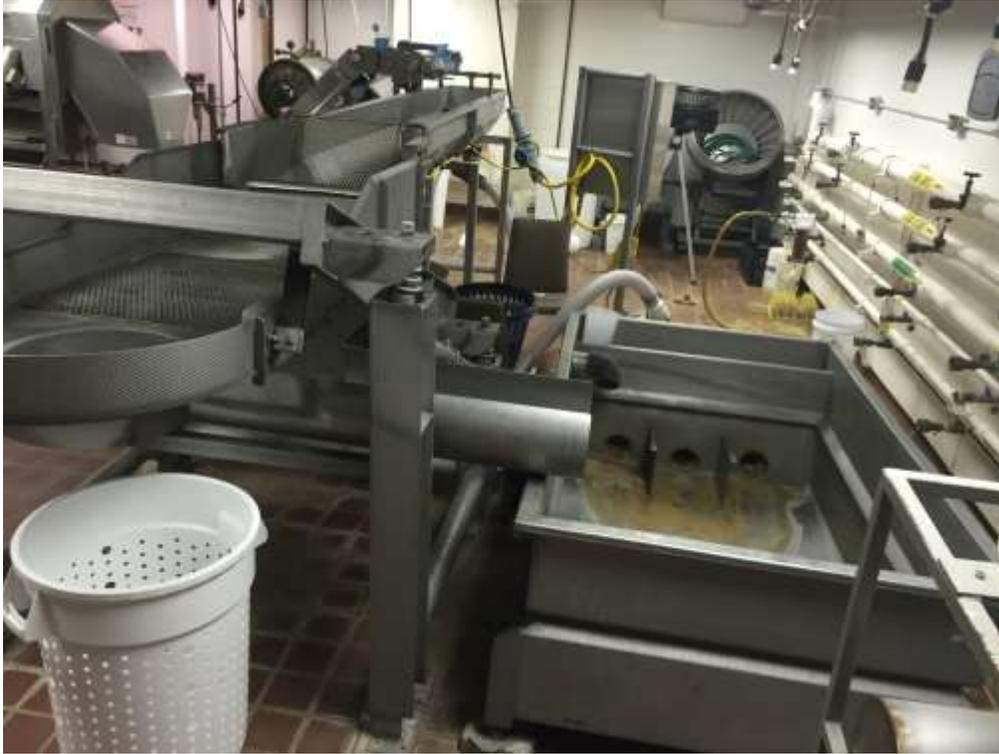
Figure 2.3: Recirculation tank
