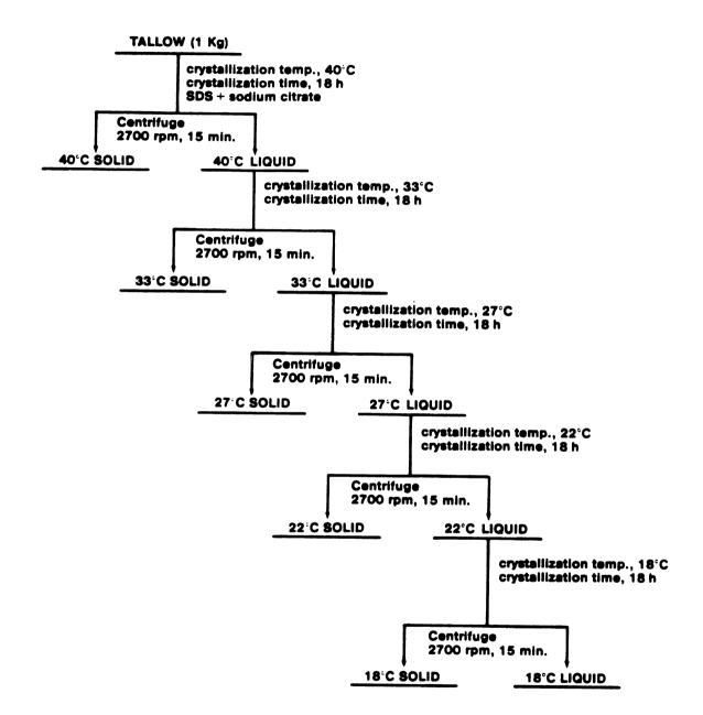
Figure 7. The modified aqueous detergent fractionation process utilized in the derivation of frying oils from refined edible beef tallow.
