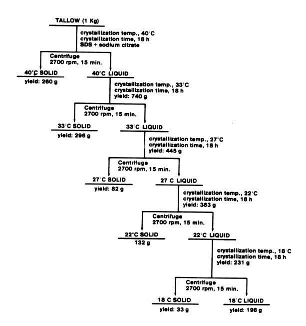
Figure 10. The fractionation scheme of edible tallow using sodium dodecyl sulfate and sodium citrate.
