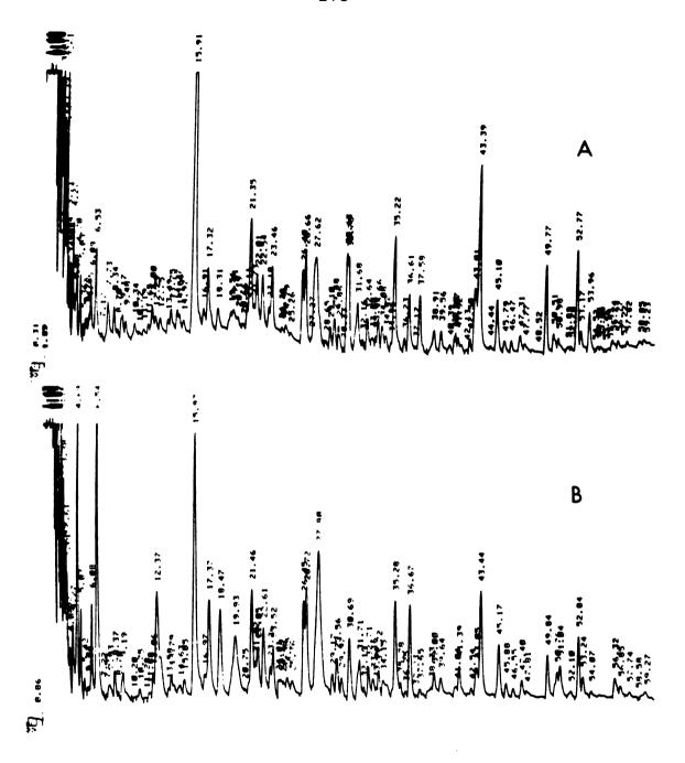
Figure 23. Capillary GC chromatograms of volatile flavor extracts of potato chips fried in 22°C olein, after storage for 0 weeks (A) and 5 weeks (B) at room temperature.
