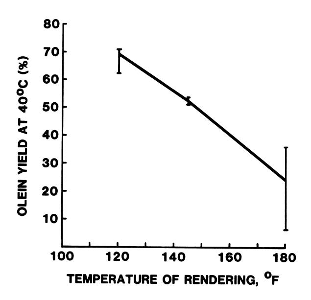
Figure 8. Olein yields of tallows fractionated at 40°C versus temperature of rendering, °F.
