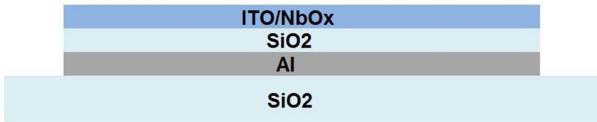
Figure 50. Full stack of ITO/NbO<sub>x</sub>, SiO<sub>2</sub>, and Al creating the basis for the capacitors/switches
