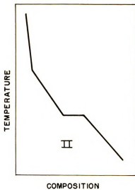
Cooling curve with eutectic halt in a two-component system.
