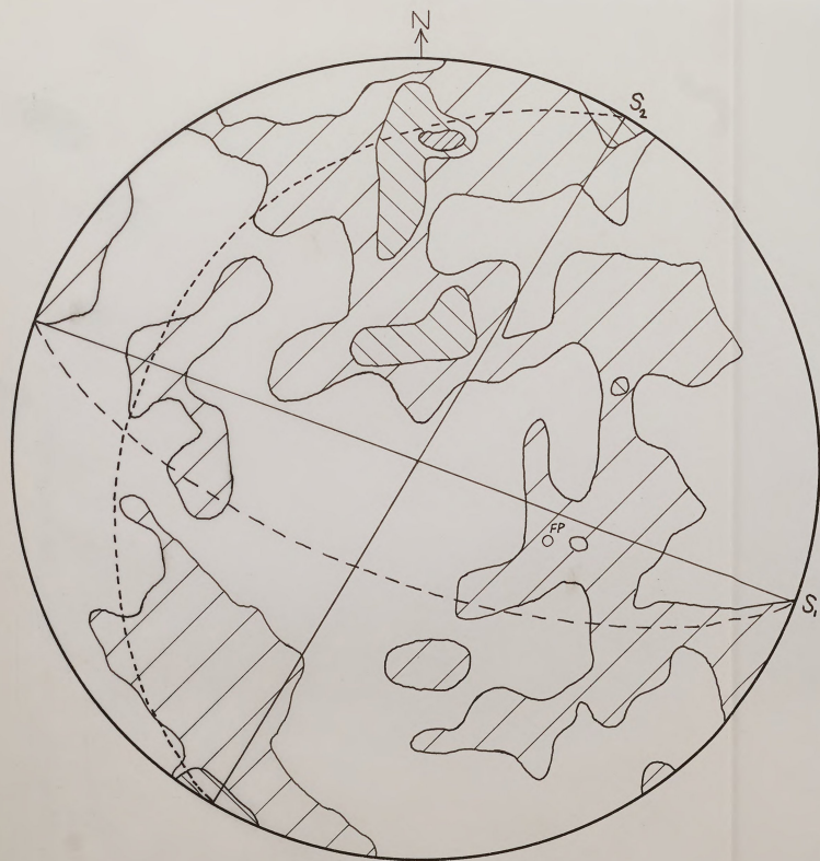
FIGURE 17. SAMPLE 15, COMBINED DIAGRAM, WALL RAVINE, CONGLOMERATIC FACIES. 400 QUARTZ C-AXES; GRAIN SIZE > .3\text{mm} . CONTOURS 3-2-1% S_1 IS THE BEDDING PLANE. S_2 IS THE FAULT PLANE. FP IS THE FACE POLE OF THE FAULT.
