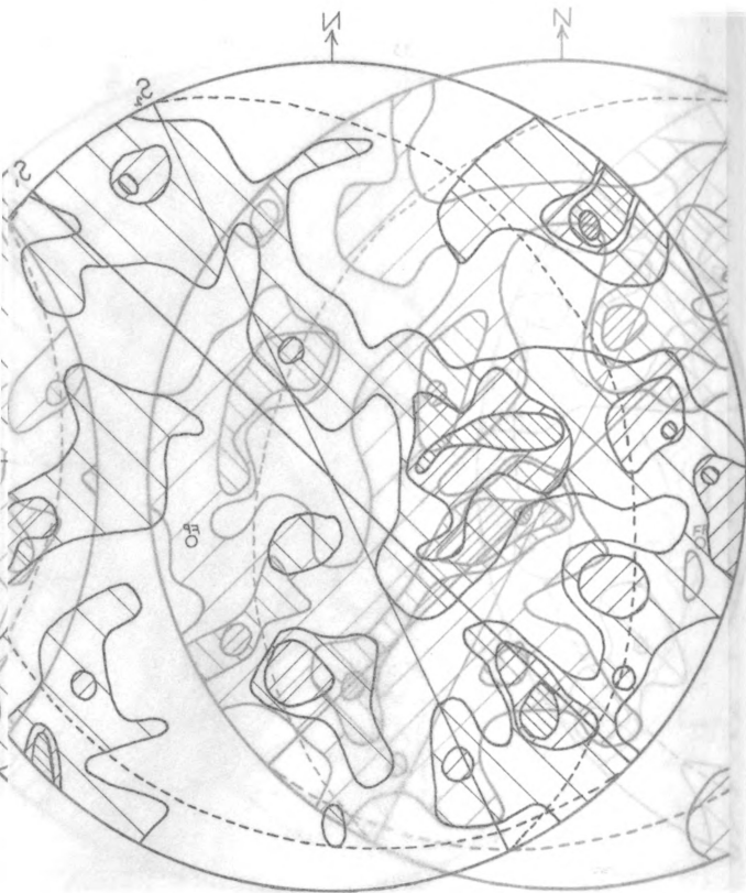
Figure 33. Sample 19, vertical cut, Saint Louis Ravine Conglomerate. The map shows the distribution of 500 Quartz C-axes (grain size > 3mm) contours 4-3-5-1. The dashed line 'S' is the bedding plane, 'FP' is the fault plane. The shaded areas are the fault zone.
