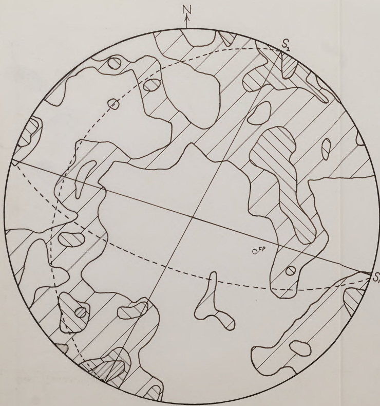
FIGURE 15. SAMPLE 15, HORIZONTAL CUT, WALL RAVINE, CONGLOMERATIC FACIES. 200 QUARTZ C-AXES; GRAIN SIZE 7-3mm. CONTOURS 3-2-1% S_1 IS THE BEDDING PLANE. S_2 IS THE FAULT PLANE. FP IS THE FACE POLE OF THE FAULT.
