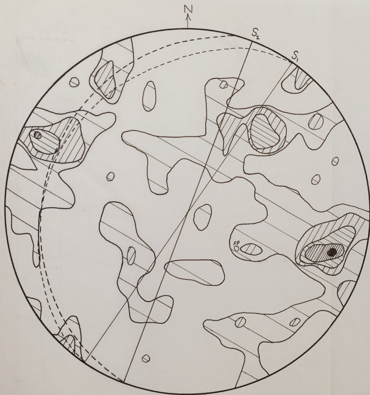
FIGURE 31. SAMPLE 1, VERTICAL CUT, DOUGLASS HOUGHTON RAVINE, CONGLOMERATIC FACIES, 200 QUARTZ C-AXES; GRAIN SIZE > 3 mm. CONTOURS 5-4-3-2-1% S_1 IS THE BEDDING PLANE. S_2 IS THE FAULT PLANE. FP IS THE FACE POLE OF THE FAULT.
