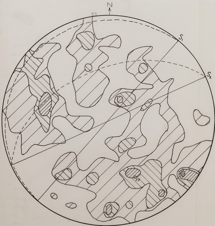
FIGURE 51. SAMPLE 20, HORIZONTAL CUT, TOBACCO RIVER, 200 QUARTZ C-AXES; GRAIN SIZE APPROXIMATELY .2mm. CONTOURS 4-3-2-1-0. S_1 IS THE BEDDING PLANE. S_2 IS THE FAULT PLANE. FP IS THE FACE POLE OF THE FAULT.
