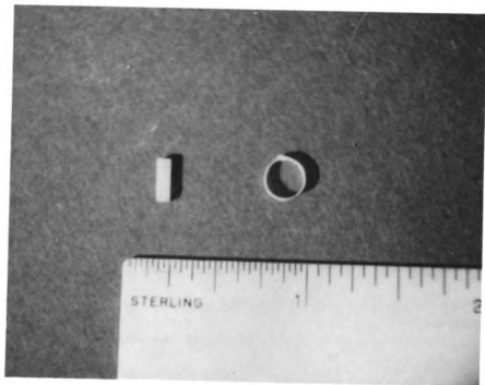
Figure 4.3 Rectangular cotyledon specimen (left) and seed coat ring specimen (right).
