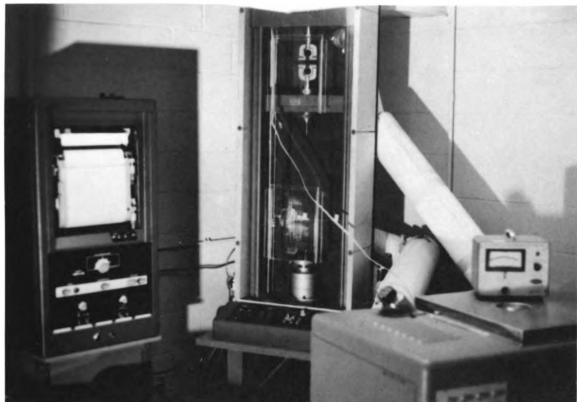
Figure 4.1 Instron Universal Testing Machine with the chamber connected to Aminco-Aire unit.
