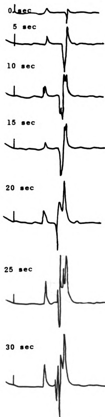
Figure 42. Examples of baseline disturbances due to refractive index change caused by mixing of heartcut solvent and developing solvent.
