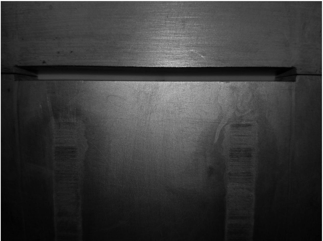
Figure A.14 Gaps on the sides of the 3D printed structure.
