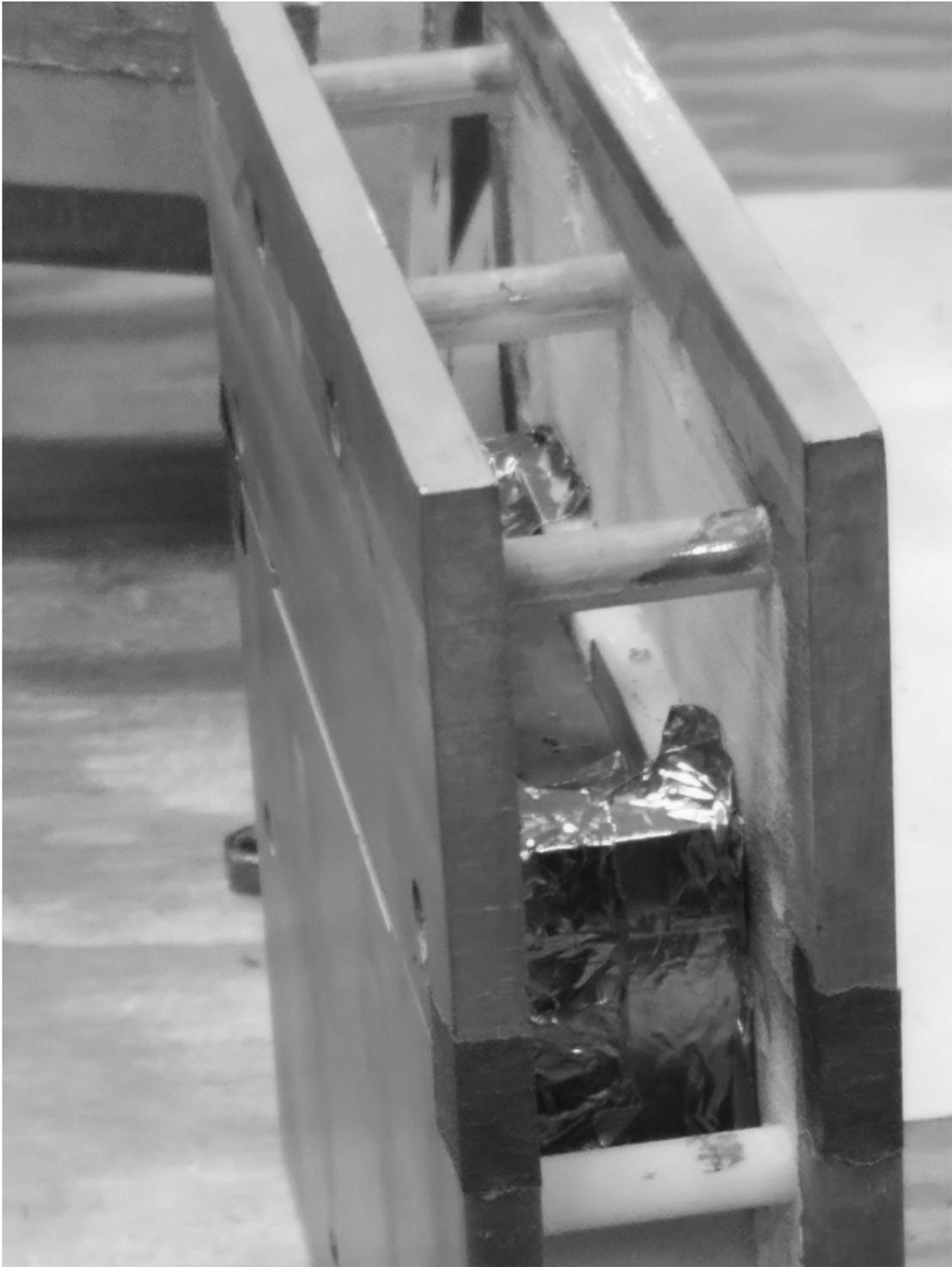
Figure A.16 Taping the sides of the 3D printed structure.
