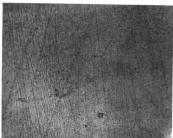
Fig. 16 Optical micrographs illustrating microstructural changes accompanying isochronal annealing of 72% cold rolled specimens:
