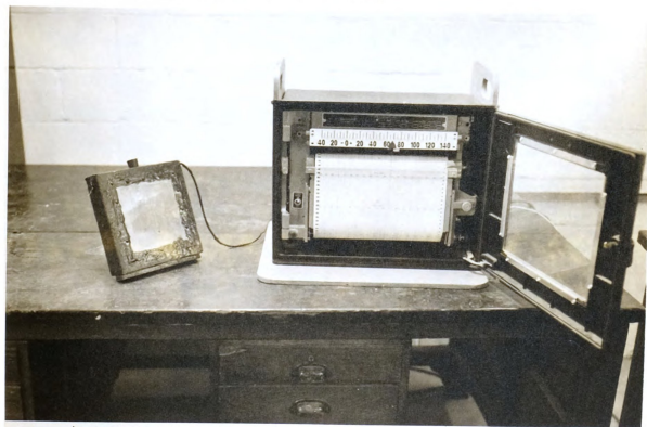
Fig. 4. Apparatus for determining the thermal diffusivity of grain.
