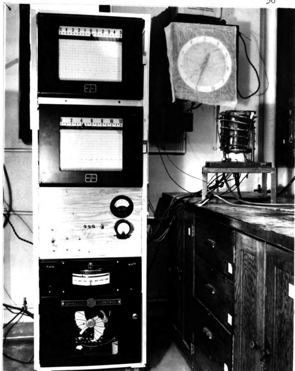
PHOTO 4. ASSEMBLY OF DIFFERENTIAL THERMAL ANALYSIS EQUIPMENT. IN THE VERTICAL MOUNT ON THE LEFT FROM THE TOP DOWN IS THE DIFFERENTIAL TEMPERATURE RECORDER, THE SAMPLE TEMPERATURE RECORDER, THE CONTROL PANEL, AND THE WHEELCO CHRONOTROL. ON THE WORK BENCH AT RIGHT IS THE FURNACE AND FURNACE BASE.
