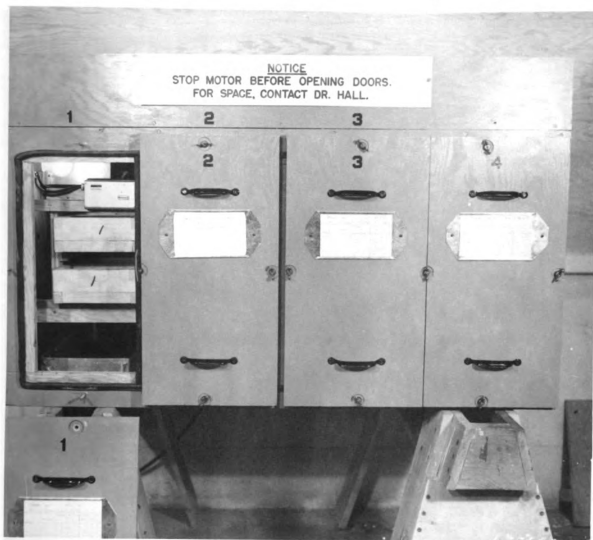
Fig. 15 Dynamic Equilibrium Moisture Chamber, showing thermostat and heating element (light bulb).
