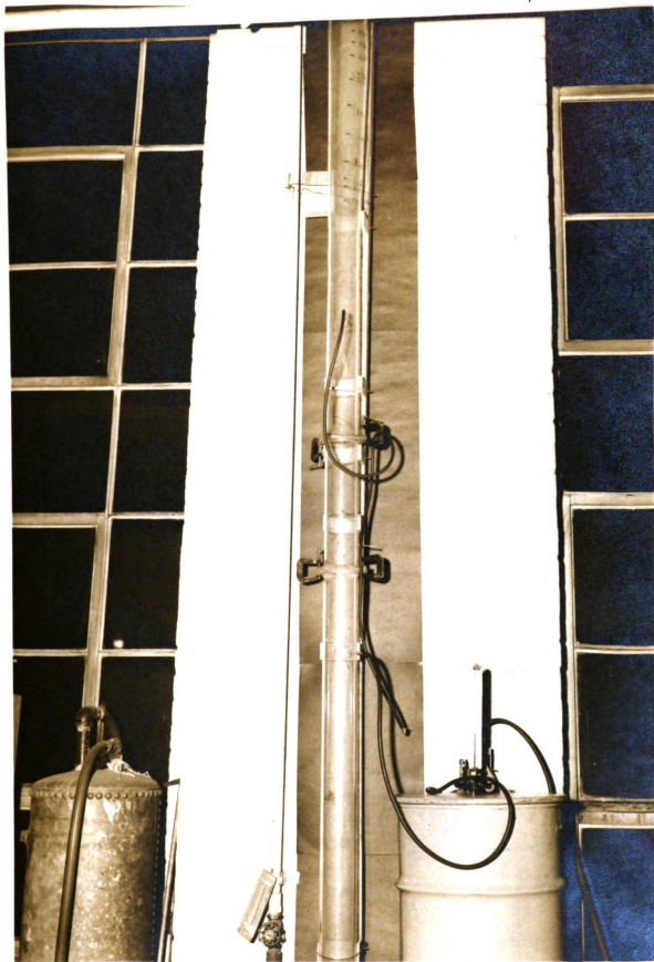
Figure 2. Apparatus used in determining suspension velocities
