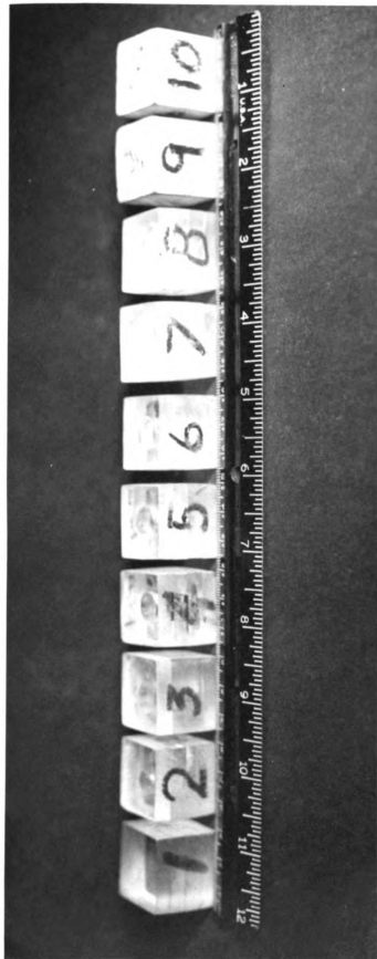
Figure 10. Some rectangular shaped particles of same size but different densities used in the tests.
