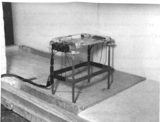
Figure 14. --Leaf model in test area of wind tunnel.
