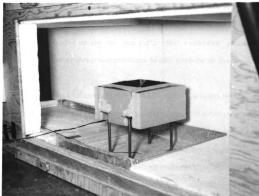
Figure 15. --Tray for measuring water application rate and drop temperature.
