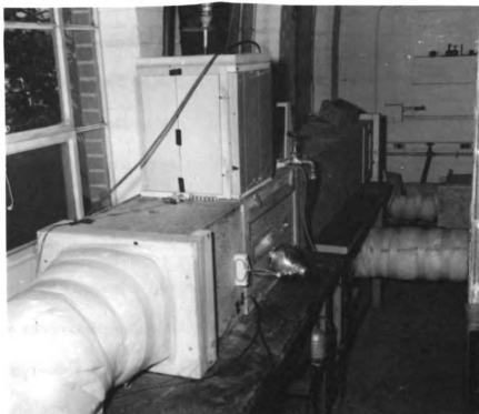
Figure 16. --Wind tunnel with sprinkling equipment attached.
