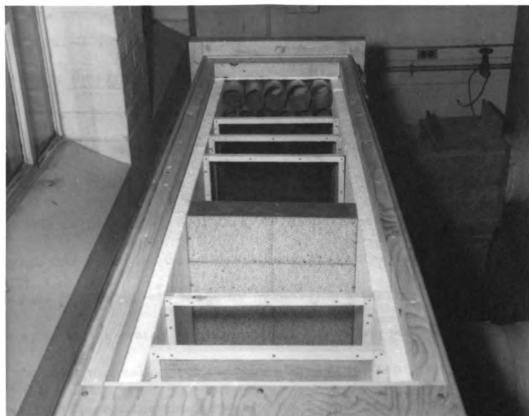
Figure 4. --Inlet section of wind tunnel.
