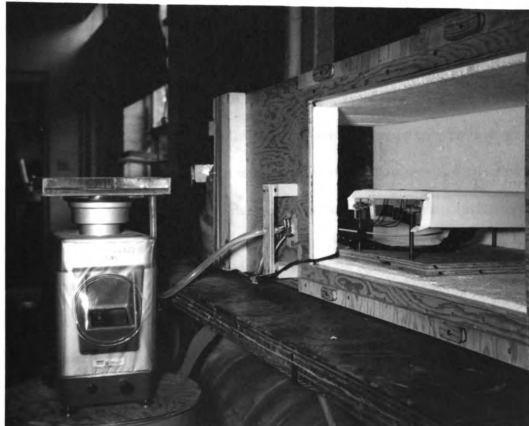
Figure 11. --Equipment set-up for measuring mass-transfer.
