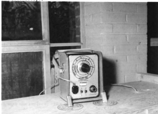
Figure 7.--Relative humidity indicator and sensors.
