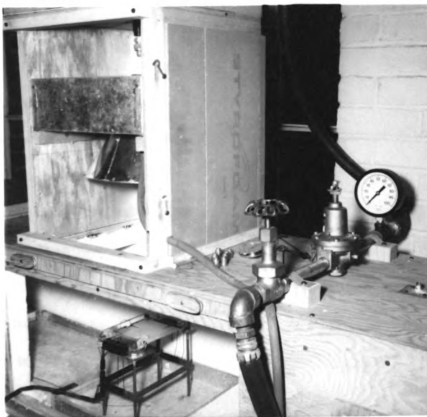
Figure 17. --Sprinkling tower and water control assembly.
