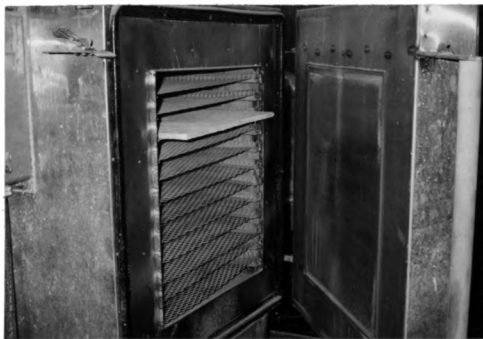
Figure 6.8 Accelerated Wetting-Drying Test Equipment.
