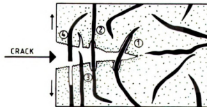
Figure 3.21 Schematic Representation of Crack Traveling Through a Fiber Reinforced Matrix [8]
