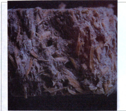
Figure 7.14 (Cont'd) Unaged Cement-Bonded Particleboard; (a) Control; (b) \text{CO}_2 -cured with southern pine used; (c) \text{CO}_2 -cured with aspen used
