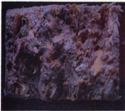
Figure 7.16 (Cont'd) After Repeated Freezing-Thawing on Cement-Bonded Particle-board; (a) Control; (b) CO 2 -cured with southern pine used; (c) CO 2 -cured with aspen used
