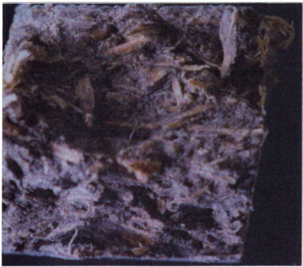
Figure 7.16 After Repeated Freezing-Thawing on Cement-Bonded Particleboard; (a) Control; (b) CO 2 -cured with southern pine used; (c) CO 2 -cured with aspen used
