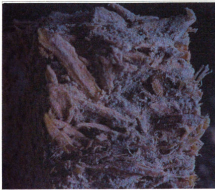
Figure 7.15 After Repeated Wetting-Drying on Cement-Bonded Particleboard; (a) Control; (b) \text{CO}_2 -cured with southern pine used; (c) \text{CO}_2 -cured with aspen used
