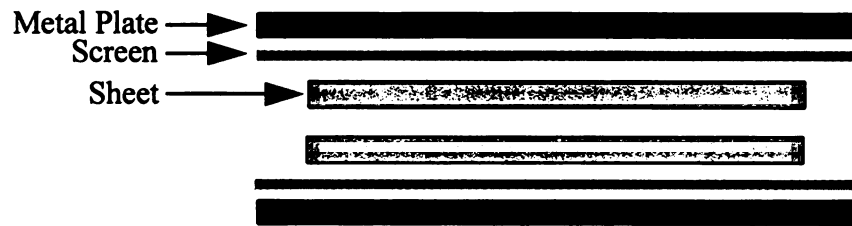
Figure 4.19 Schematic of Formation of Two-Ply Cellulose Fiber Reinforced Cement Composite Sheet
