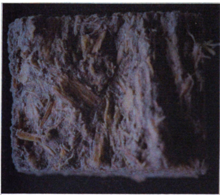
Figure 7.14 Unaged Cement-Bonded Particleboard; (a) Control; (b) CO 2 -cured with southern pine used; (c) CO 2 -cured with aspen used
