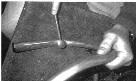
Figure 214 Hammering wrinkles out of formed bottom bow
