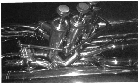
Figure 224 Linkage for fifth valve — A
