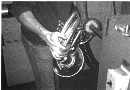
Figure 227 Polishing the instrument on buffing machine — B
