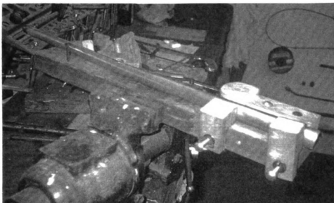
Figure 212 Jig for bending bottom bow
