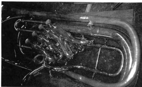
Figure 215 Bottom bow attached to bass trombone bell, spot-soldered in approximate position
