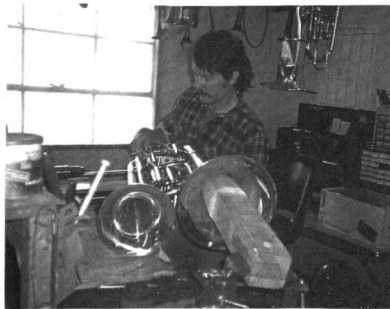
Figure 223 Installing branch to rotary valve
