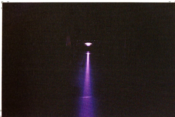
Figure 9.10(b) 2 electrode system, 10.0 kV, 0.84 cm separation.
