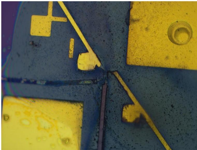
Figure 3.30: Etched surface by ionic liquid after the measurement. The liquid dispersed all over the surface.
