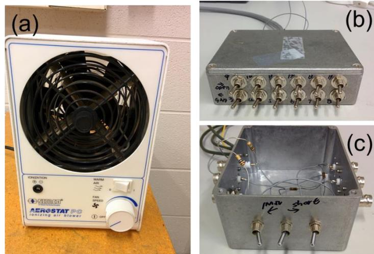
Figure 3.14: Other anti-ESD apparatus. (a) Ion fan (b,c) grounding switch boxes for turning on/off grounding on each probe/channel. The buffer resistors used in the box are  $1\text{M}\Omega$  for each channel.
