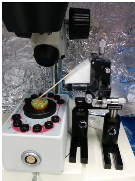
Figure 3.24: The toothpick attached on the optical microstage used in dipping ionic liquid on the chip.
