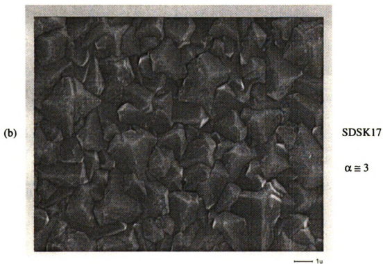
Figure 6.23. SEM pictures of \{111\} films with (a) rough faces and (b) smooth faces.
