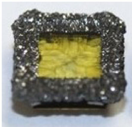
Figure 2.20 The seed substrate plus the synthesized diamond after 35.5 h of deposition time. [67]
