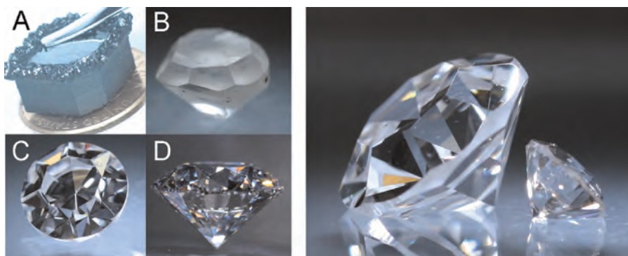
Figure 2.16 The picture on the right shows a 2.4 carat single crystal diamond CVD diamond compared with 0.25 carat CVD diamond. Example of the evaluation of CVD diamond single crystal starting with crystal 13.5 carat block (A) to the 2.3 carat cut anvil (D). [66]
