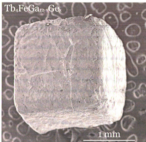
Figure IV.1. SEM image of a typical Ga-grown \text{Tb}_4\text{FeGa}_{12-x}\text{Ge}_x crystal. The roughening of the surface is caused by an etching process during isolation.
