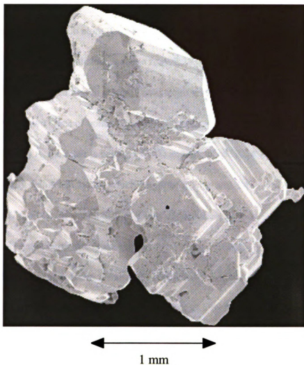
Figure 5-1 Scanning electron micrograph of \text{Tm}_5\text{Co}_4\text{Si}_{14} crystal clusters. This figure shows the crystal habit and plate stack twinning typical of these compounds.
