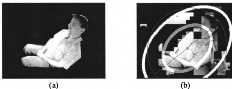
Figure 2.9: Marker regions for watershed processing for the occupant shown in Figure 2.7, (a) hand segmented image, and (b) inner and outer marker regions.
