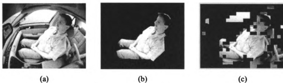
Figure 2.7: Demonstration of artifacts to be reduced by post-processing, (a) original image, (b) desired segmentation, and (c) output from the background subtraction-based segmentation.
