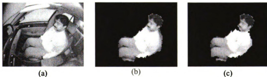
Figure 6.27: Example of correct adult segmentation, (a) raw image, (b) preliminary segmentation, and (c) final random mutation blob combining segmentation output.
