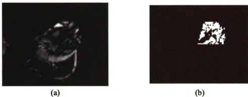
Figure 7.29: Images for Hausdorff pre-processing, (a) difference image, and (b) thresholded and region limited difference image.
