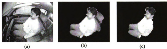
Figure 6.20: Example of correct adult segmentation, (a) raw image, (b) preliminary segmentation, and (c) final forward sequential search segmentation output.
