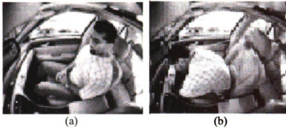
Figure 5.3: Demonstration of need for history algorithm, (a) adult seated normally, and (b) adult leaning forward and appearing to system to be an infant in a RFIS.
