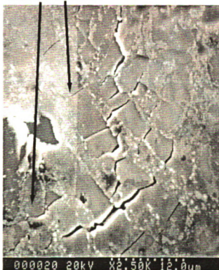
Figure 6.2. Higher magnification SEM micrographs of room temperature creep specimen after 0.05 strain from (a) center and (b) right regions of the joint. Both regions reveal microcracks and (a) shows grain rotation and shearing perpendicular to \text{Ag}_3\text{Sn} particle bands.
