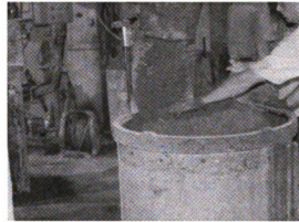
Figure 3.6. Pouring of Concrete into Mold
