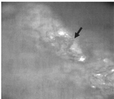
Figure 32: Metallic Polish from Cutting Dry Reed (artifact no. 52, 300X)
