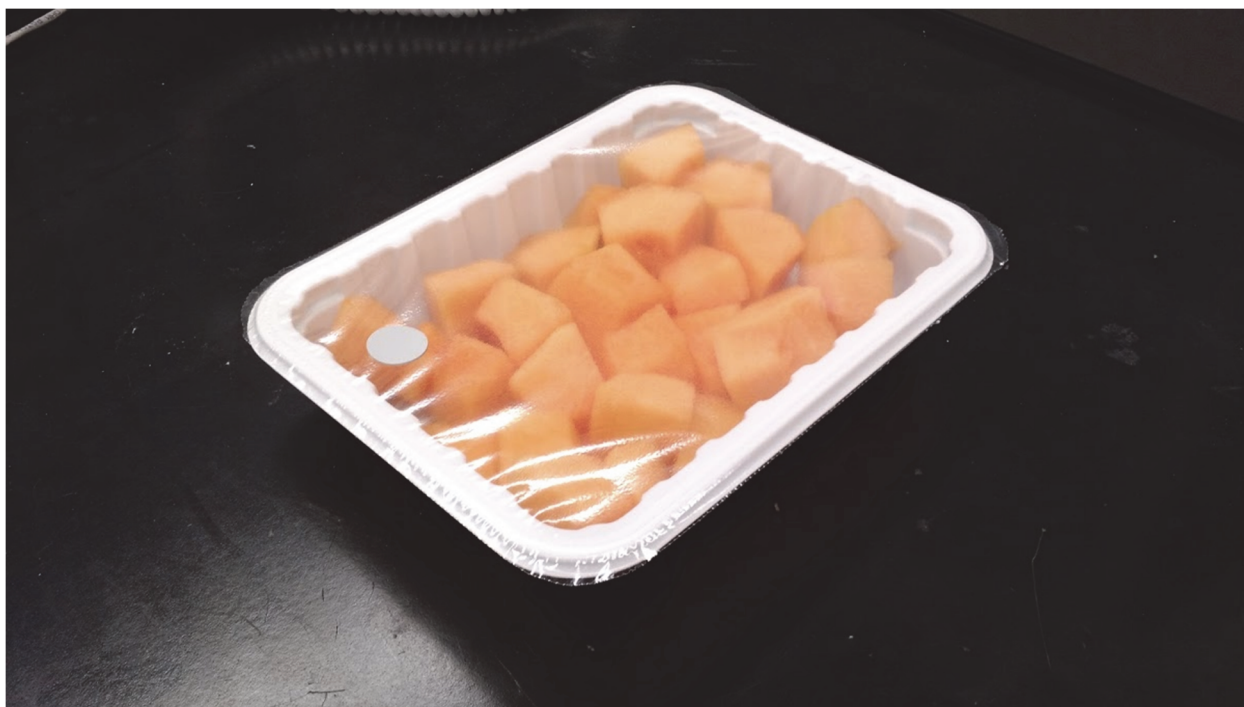
Figure 3. Package of fresh-cut cantaloupe, with adhesive septum for headspace gas extraction
