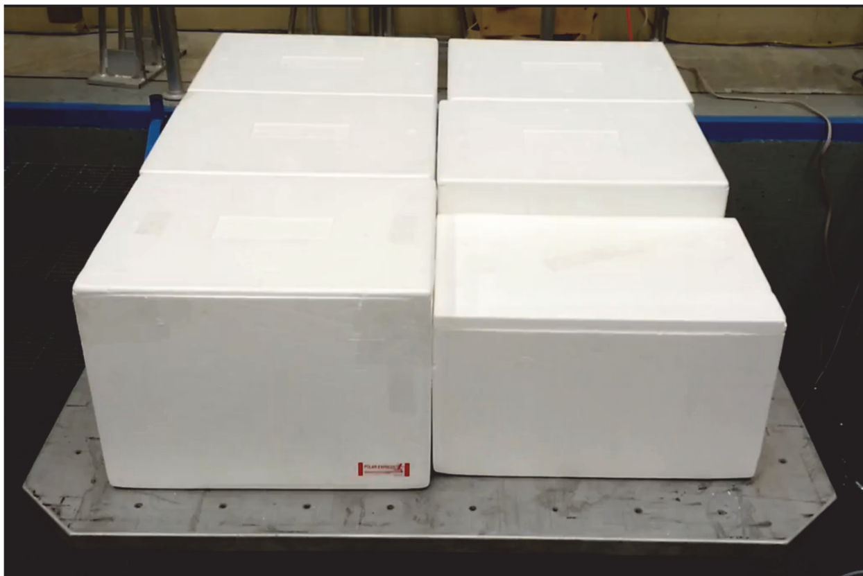
Figure 4. Vibration table with attached EPS coolers.
