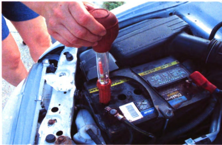
Figure 103 Squeeze the Bulb and Insert the Hydrometer
