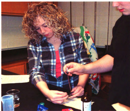
Figure 124 Using Capillary Action to Introduce the Electrolyte
