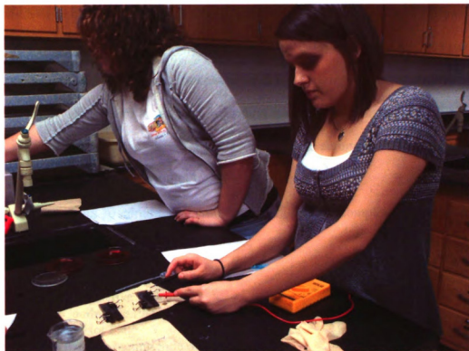
Figure 125 Testing Current and Voltage Output of the Finished PV Cells
