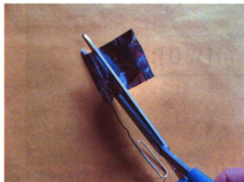
Figure 89e After rolling the foil around match and clip a few times, cut the excess foil off.
