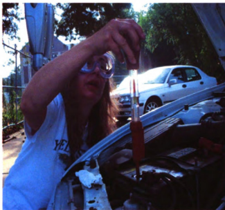
Figure 104 Reading Specific Gravity Value
