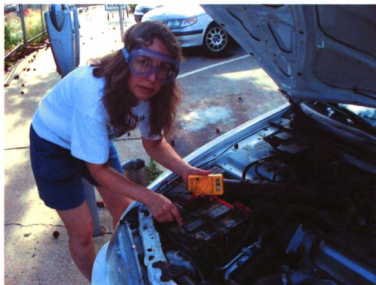
Figure 99 Testing Voltage on a Car Battery
