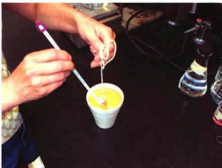
Figure 84 Heat Lost by the Metal is Gained by the Liquid
