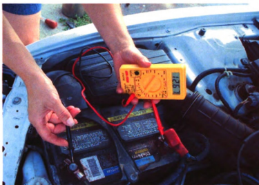
Figure 100 Close-Up of Testing Voltage on a Car Battery
