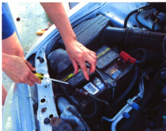
Figure 101 Prying Caps Off the Battery Cells
