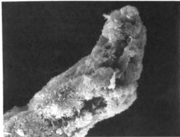
Figure 6.2.--Electron scanning microscope photographs of partially decomposed fibers. (a) Nutrient, bacteria, and a crack. (b) Cavities inside the fiber. (c) Cavity along the length of the fiber. (d) A complete split of the fiber. (e) Advanced stage of decomposition with loss of structural integrity.
