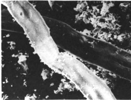
Figure 6.1.--Electron scanning microscope photographs. (a) Undecomposed cellulose fiber. (b) Undecomposed cellulose with Kaolinite particles.
